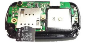
(  $\rm I$  ) Open the top cover with the screw driver, Insert a mini SIM card support GSM/GPRS network into the slot and make sure the chip side is down.
