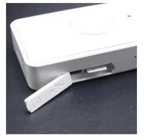
5.2 Install the SIM card correctly that to active device)
